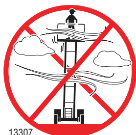
13307 DO NOT ELEVATE IN WINDY CONDITIONS
