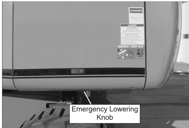
Figure 4.3 – Emergency Lowering Knob
