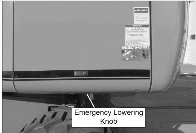
Figure 10.5 – Emergency Lowering Knob
