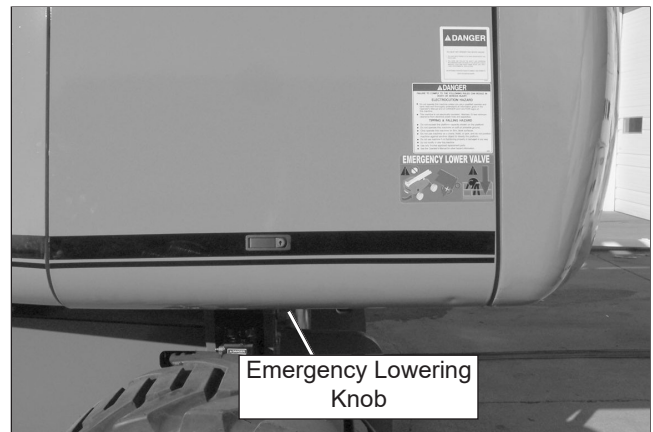
Figure 7.8 – Emergency Lowering Knob
