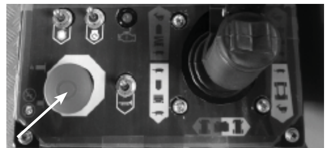
Figure 8.2 - Emergency Stop switch at Platform Control Box
