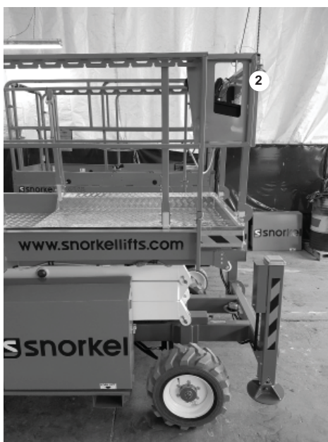
Figure 6.1.2 Control Box Location, Platform Position
