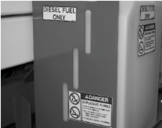
Figure 4.3 - Diesel Fuel Level
