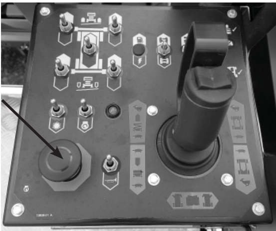
Figure 2.1 - Platform Control Box Emergency Stop Switch
