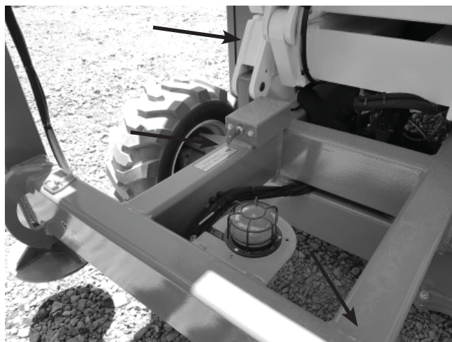
Figure 7.19 - Structural Damage and Welds
