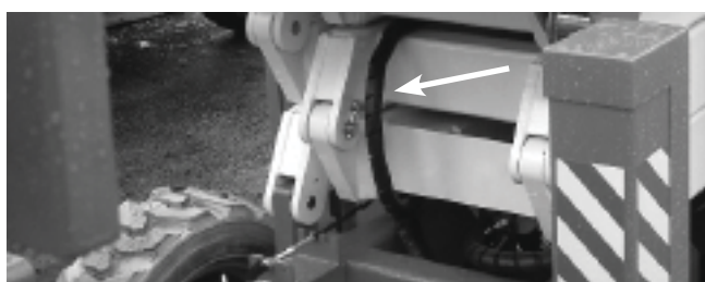
Figure 7.11 - Wiring Harness in the Scissor Stack
