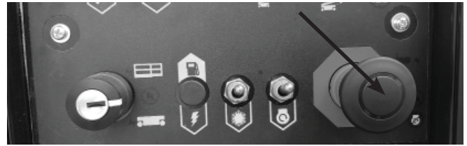
Figure 2.2 - Ground Control Box Emergency Stop Switch
