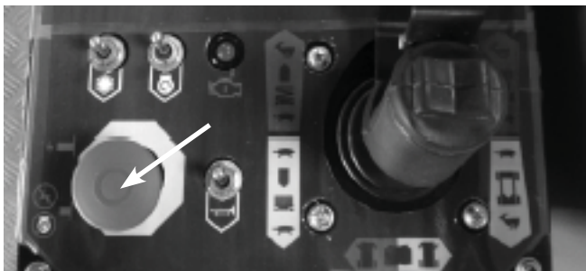
Figure 9.1 - Platform Control Box Emergency Stop Switch
