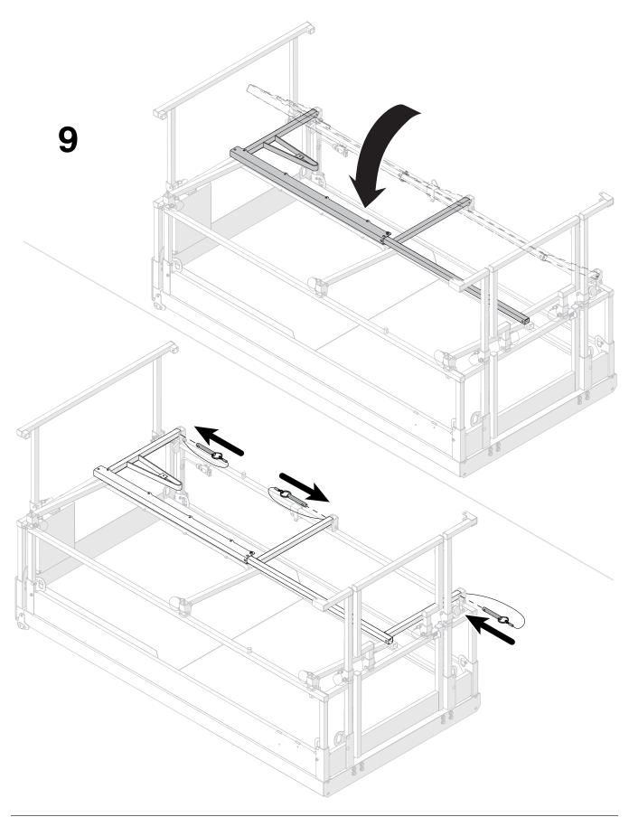
Section 6 - Procedures Fold the guardrails
