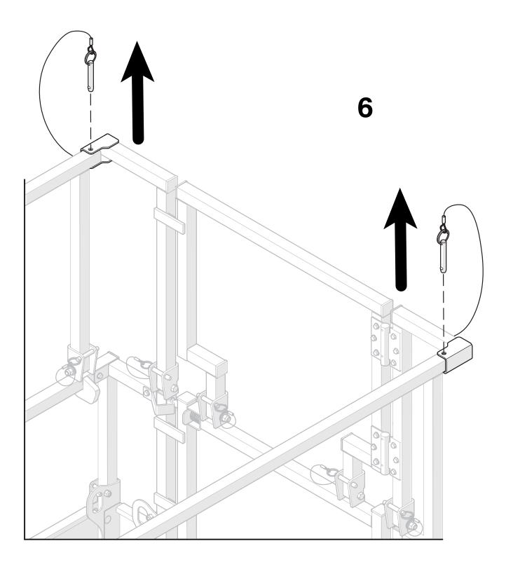
Fold the guardrails Section 6 – Procedures
