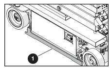
Pothole protection: This device consists of a pair of mechanically actuated guard bars located under the base. These guards automatically deploy to reduce the ground clearance when elevating the MEWP. If the pothole-protection device has not fully deployed when the MEWP is in the elevated travel position, the drive function will be disabled.
