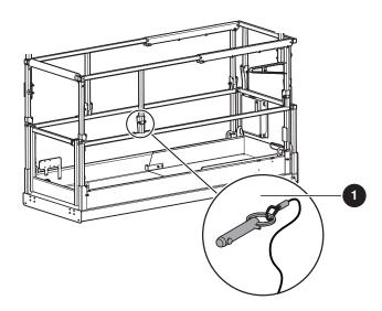
**1** Guardrail lock pin with lanyard: Use this pin to lock the guardrails. Refer to Section 6.8.
