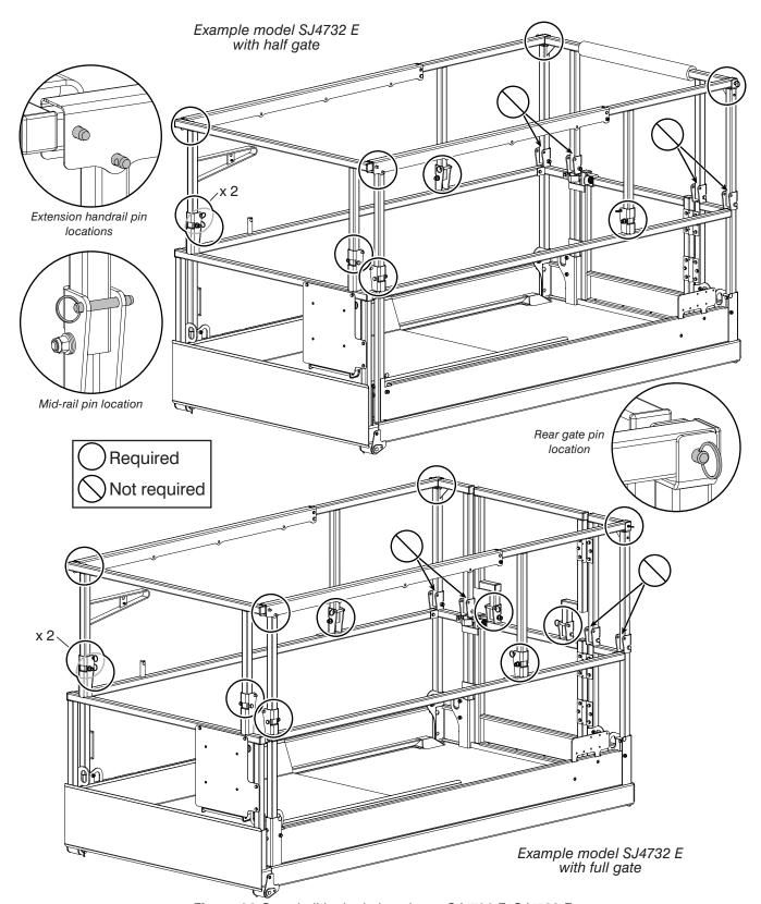
Figure 06 Guardrail lock-pin locations - SJ4726 E, SJ4732 E
