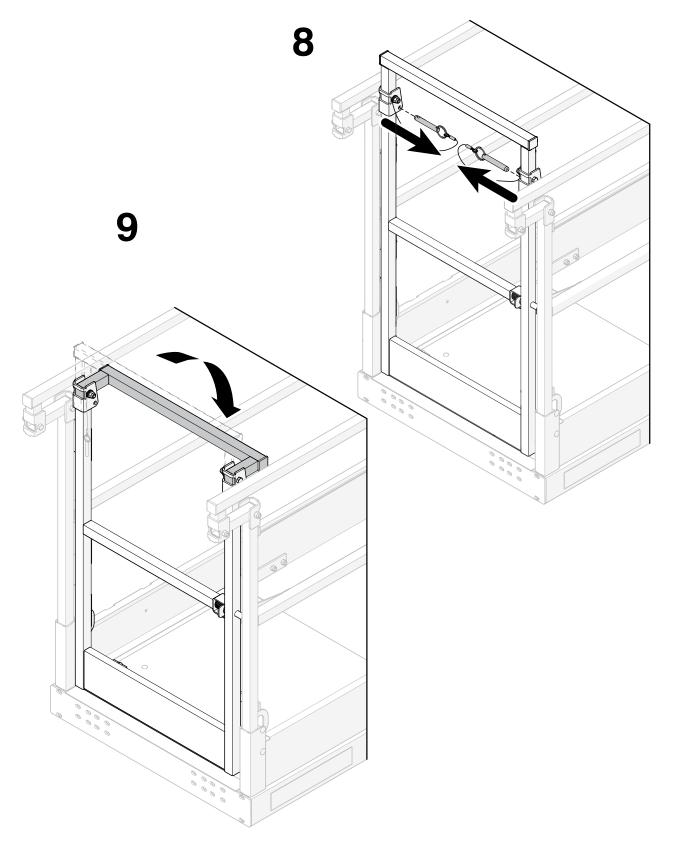
Section 6 – Procedures Fold the guardrails
