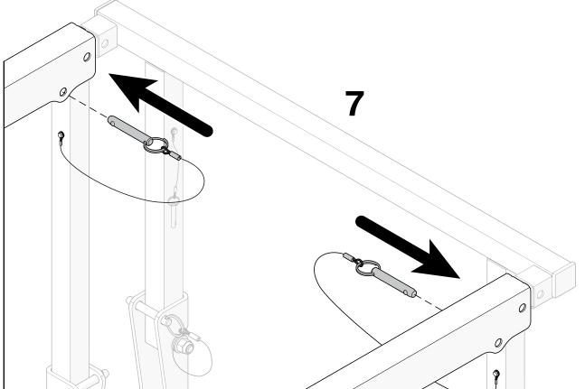
Section 6 - Procedures Fold the guardrails
