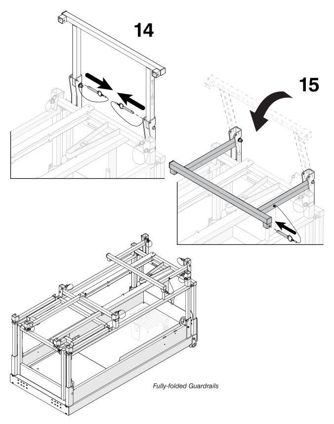
**6.** Follow the same steps shown in the illustrations in *Section 6.9* in reverse (Step 15 to Step 1) to unfold the guardrails.
