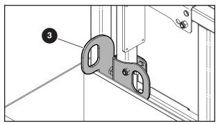
3 Fall-protection anchorage: When required, use this as a point to attach personal fall protection equipment (PFPE). Do not attach the PFPE to any other points on the platform. Do not use this anchorage to lift, anchor, attach, or hold the platform or other apparatuses or material.
