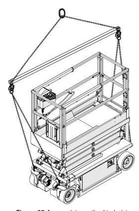
Figure 02 Appropriate method to hoist
