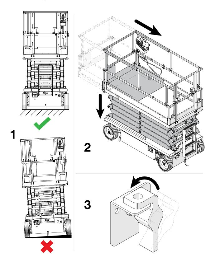
Section 6 - Procedures Fold the guardrails
