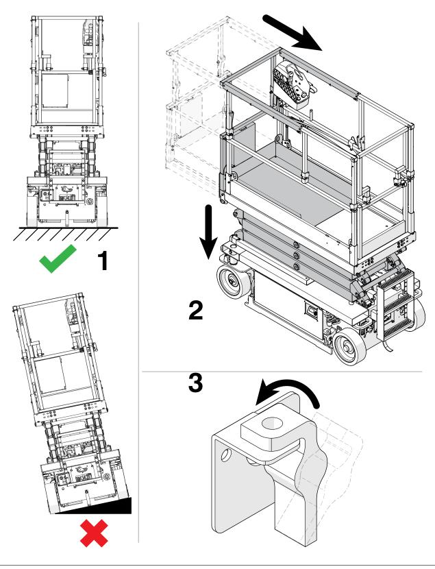
Section 6 - Procedures Fold the guardrails
