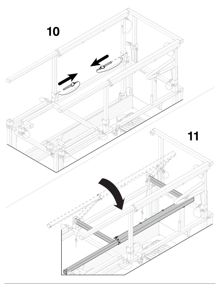
Section 6 - Procedures Fold the guardrails
