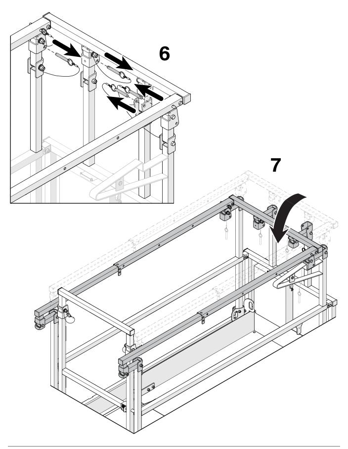
Fold the guardrails Section 6 - Procedures
