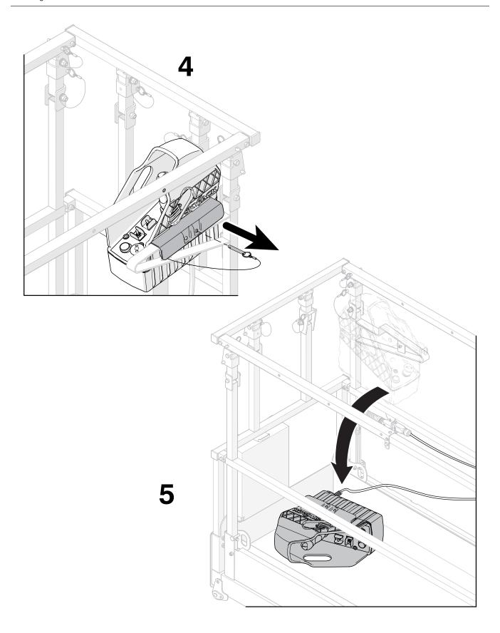
Section 6 - Procedures Fold the guardrails
