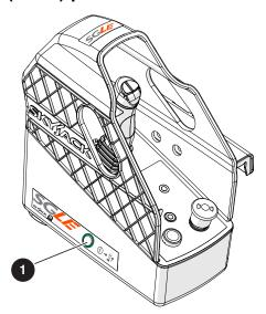
**SGLE:** This push-button energizes the lift function. Hold the button down together with the function-enable switch to enable the lift function from the platform.
