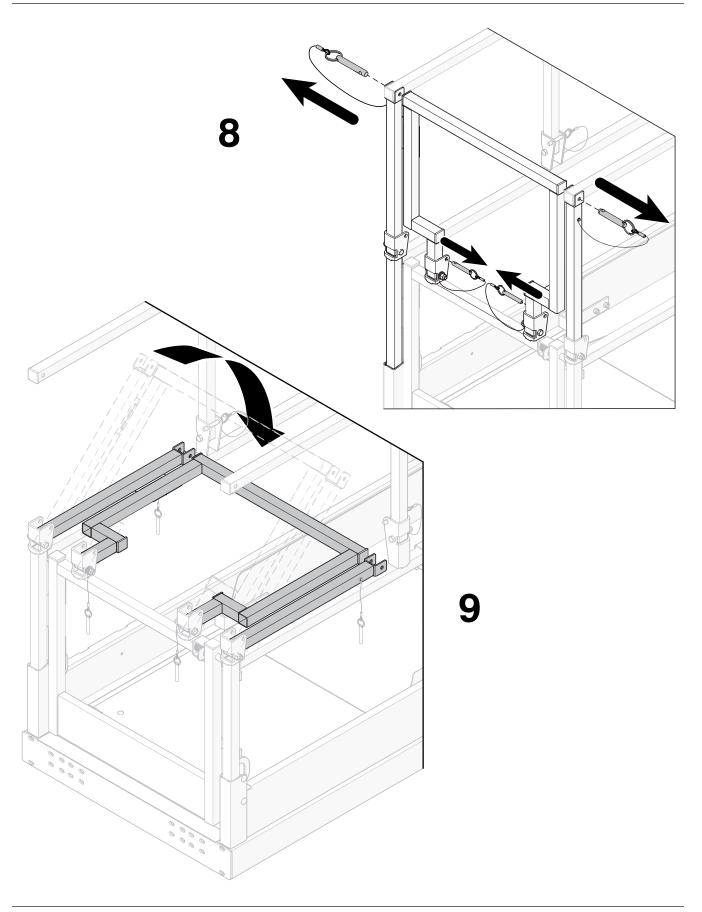
Fold the guardrails Section 6 – Procedures
