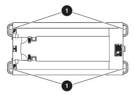
Figure 01 Lift and tie-down points
