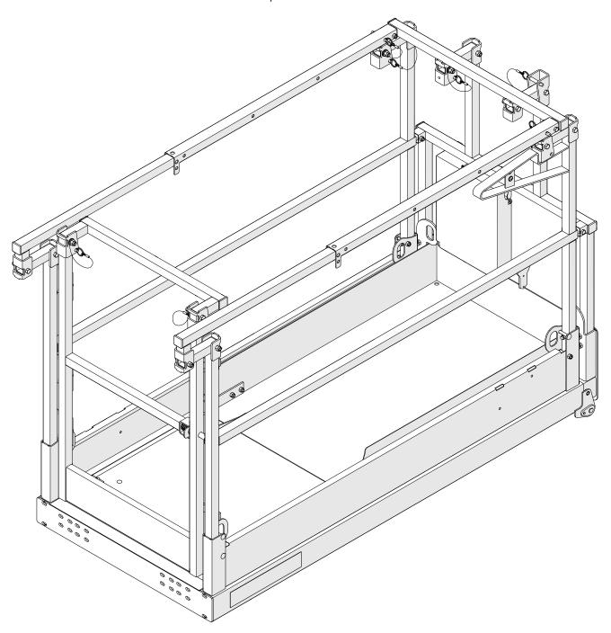
1. Follow the same steps shown in the illustrations in Section 6.9-2 in reverse (Step 9 to Step 1) to unfold the rapidfold guardrails.
