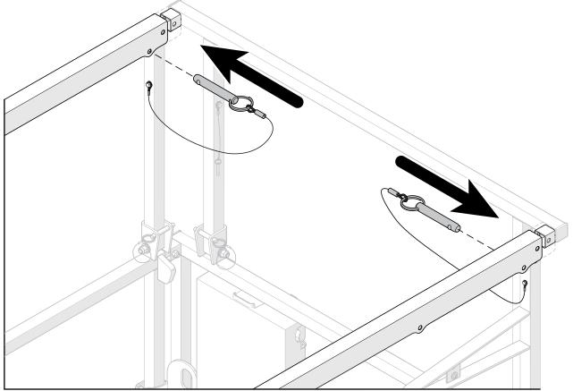
Section 6 – Procedures Fold the guardrails
