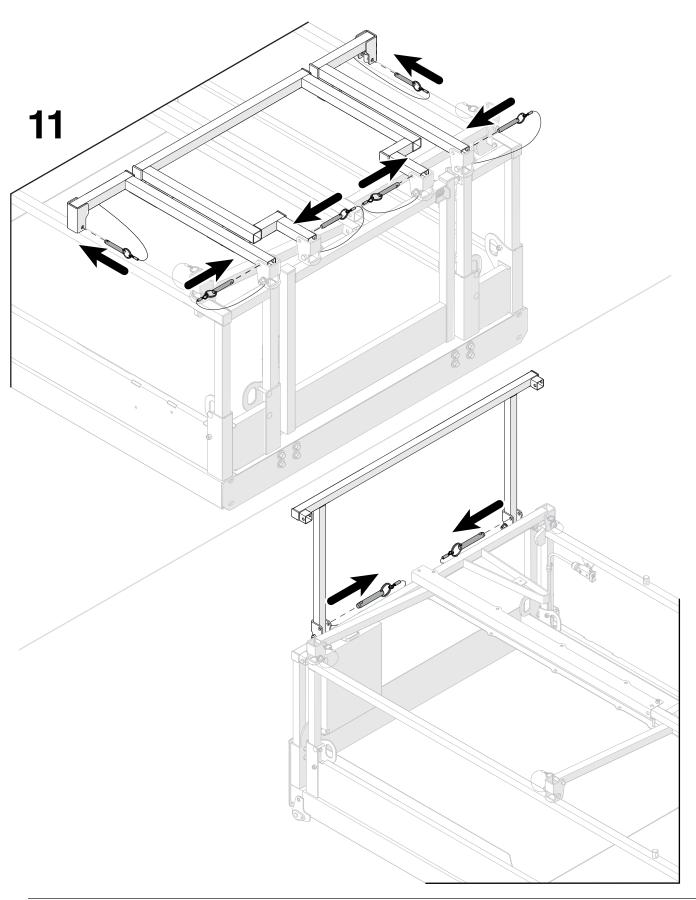
Section 6 – Procedures Fold the guardrails
