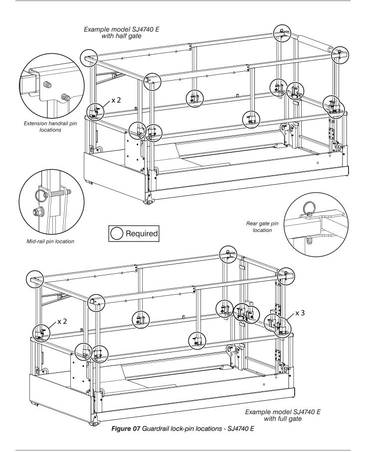
Section 6 – Procedures Fold the guardrails
