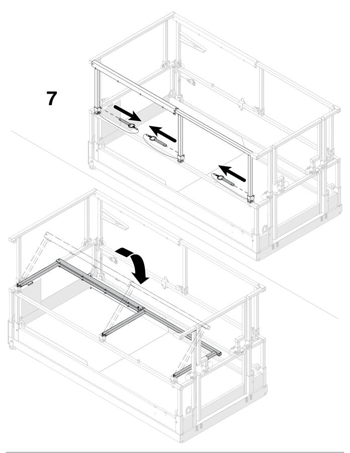
Section 6 - Procedures Fold the guardrails
