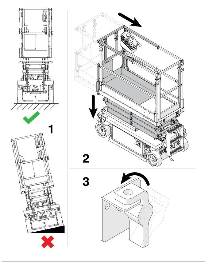
Fold the guardrails Section 6 - Procedures
