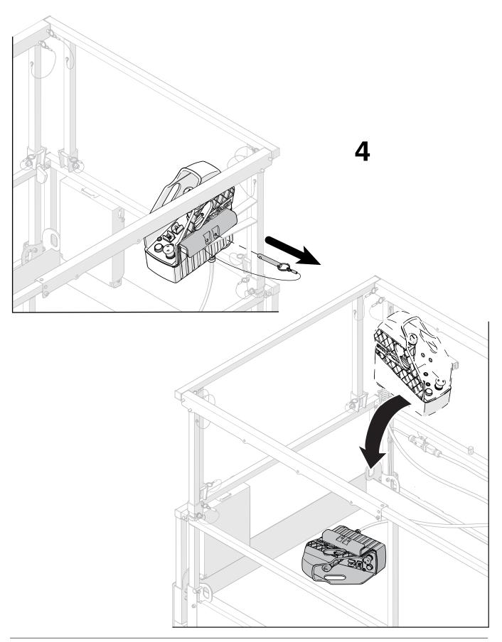
Fold the guardrails Section 6 - Procedures
