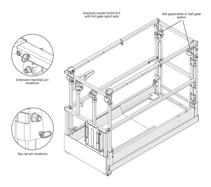
Figure 05 Rapidfold Guardrail lock-pin locations - SJ3219 E
